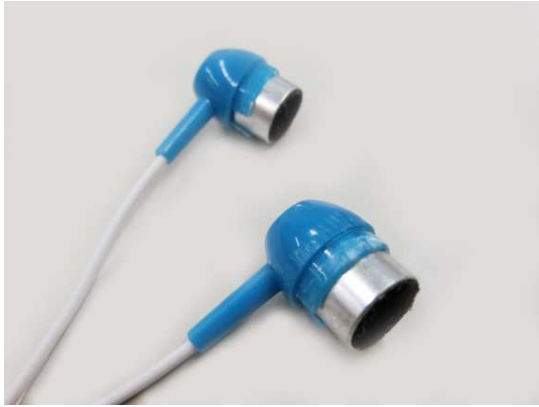
Fig. 1 Handmade binaural microphones.
