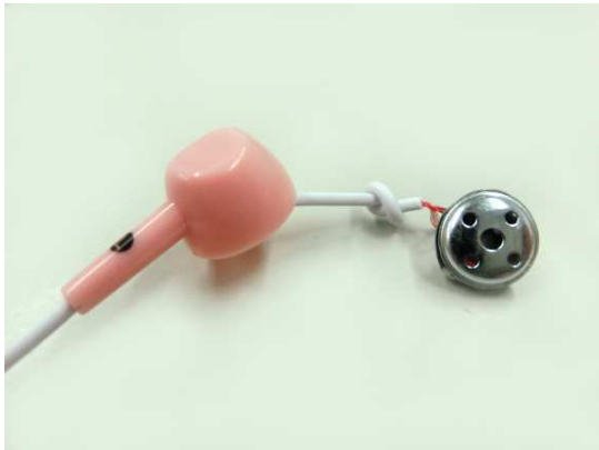
Fig. 2 A driver unit pulled out from a housing of headphones.
