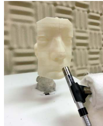
Figure 2: Physical nasal and paranasal tract model of a female subject during silent nasal breathing.
