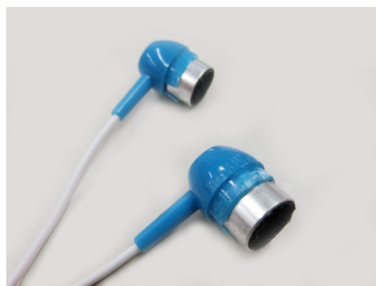
Fig. 2 Handmade binaural microphones [2].
