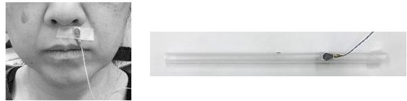
Fig.1 Acceleration sensors attached on the upper lip of participant (left) and straw (right).
